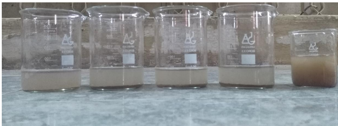
Figure 4.11: Photo of water sample after addition of 1g of crude, S4, S8, S16 and pure turbid water sample (from left to right)- after passage of 20 minutes
